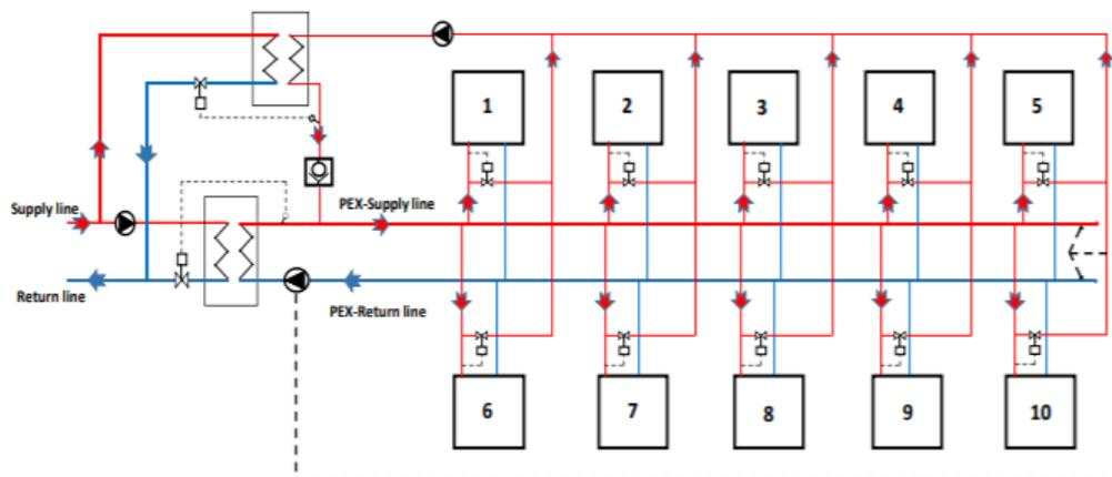
Figure 13 Connection of low-temperature network to high-temperature DH system via heat exchangers [43]
