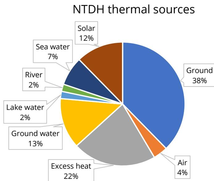
Figure 59 Overview of thermal sources in existing NTDH networks
