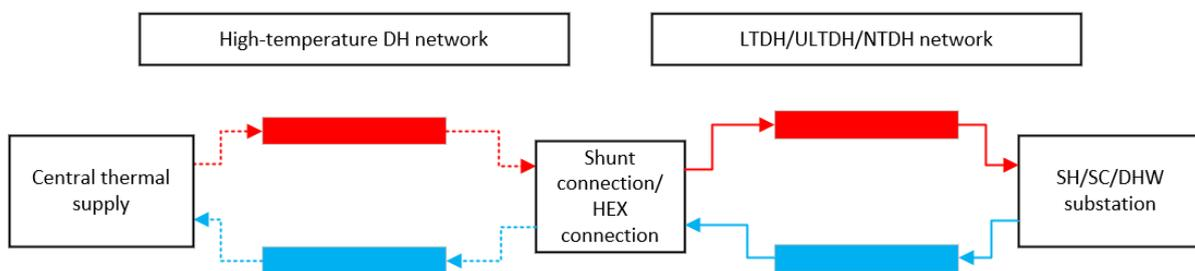
*Figure 85 Thermal sub-network – traditional DH system serves as a heat source for LTDH/ULTDH/NTDH network*
