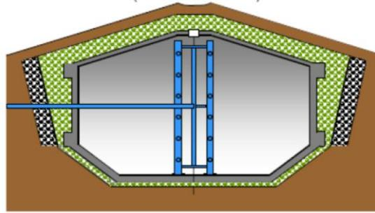
Figure 19 Tank thermal storage overview
