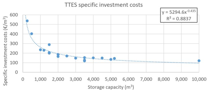
Figure 20 Tank thermal storage specific investment
