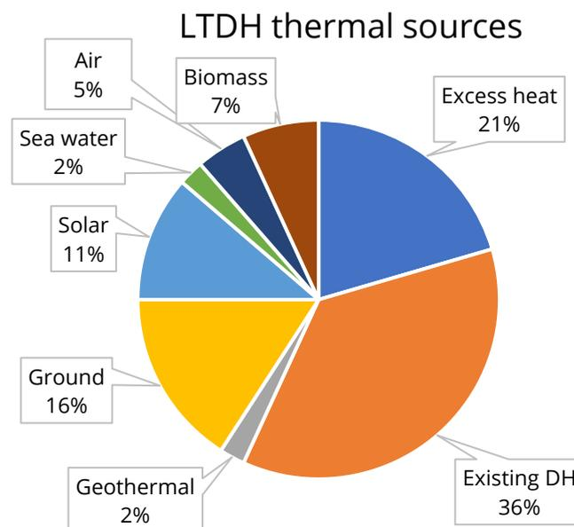
Figure 63 Overview of thermal sources in existing LTDH networks
