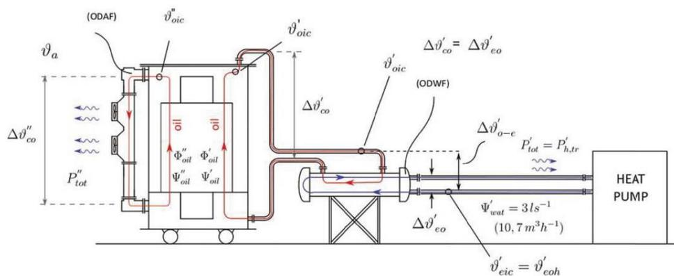
Figure 7 Power transformer waste heat utilisation scheme [26]
