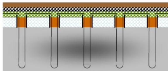
Figure 23 Borehole thermal storage overview
