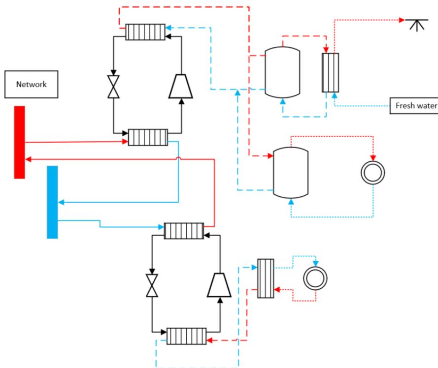
Figure 79 NTDH substation – booster heat pump for SH/DHW and heat pump for SC
