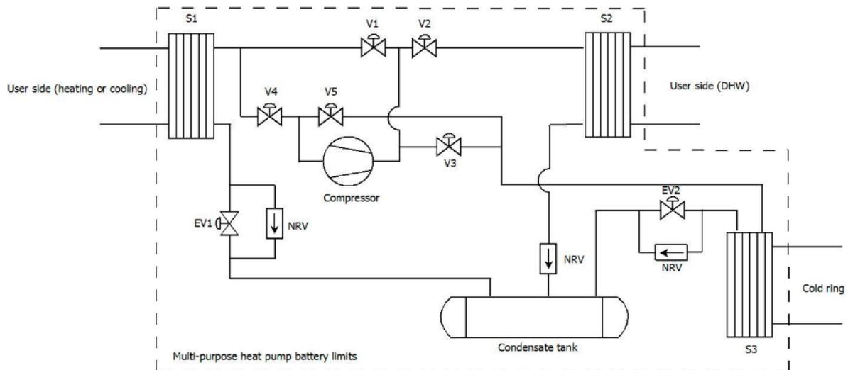
Figure 56 NTDH substation proposal [3]
