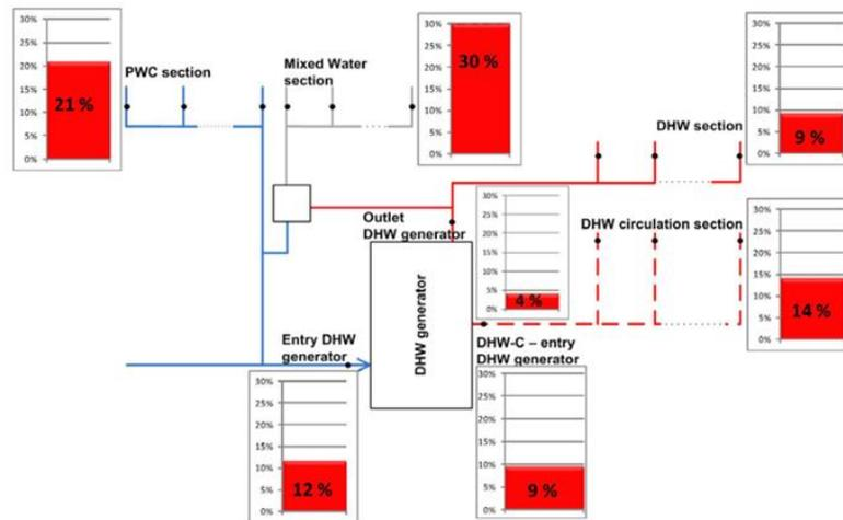
Figure 45 - Summary of central systematic and partly central contamination (K100-indications); PWC-portable water (cold); DHW-domestic hot water; blue lines-portable water, red lines-domestic hot water, grey lines-mixed water [42]
