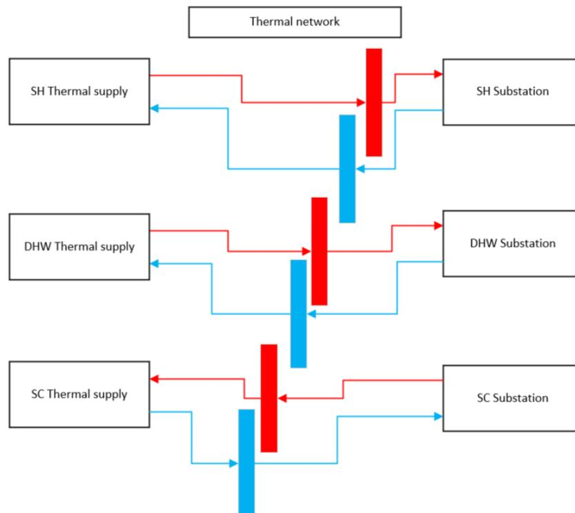
Figure 83 Thermal network – 6-pipe network for SH, SC and DHW
