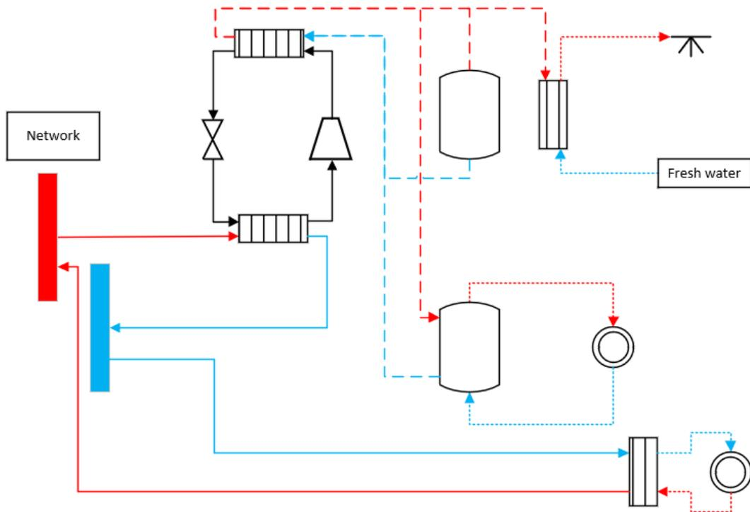
Figure 74 NTDH substation – BHP for DHW and SH, SC directly
