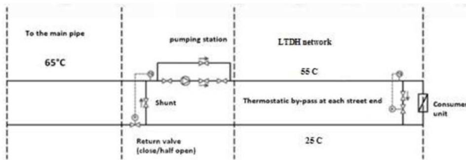
Figure 14 - Mixing shunt between existing DH and secondary network [42]
