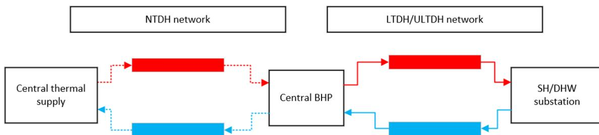
Figure 86 Thermal sub-network – NTDH serves as a heat source for LTDH/ULTDH network
