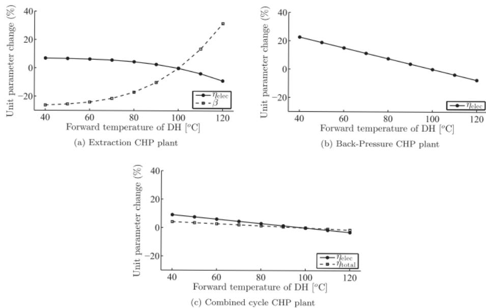
Figure 11 The impact of supply temperature reduction on various CHP types [6]
