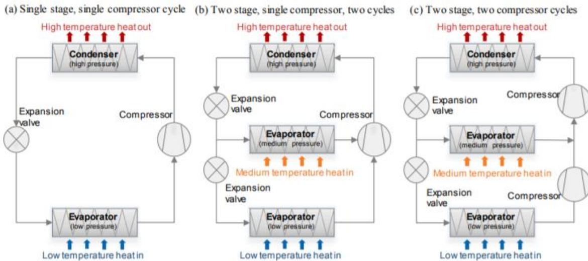
Figure 4: Potential thermodynamic cycles for upgrading data centre waste heat (a) Single stage, single compressor cycle (b) Two-stage, single compressor, two cycles (c) Two-stage, two compressor cycle
