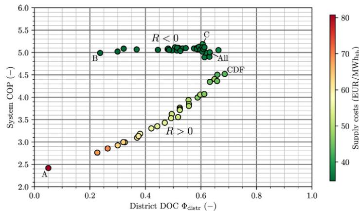
Figure 41 The impact of heating and cooling simultaneousness (DOC) and heating-cooling ratio ( $R$ )
