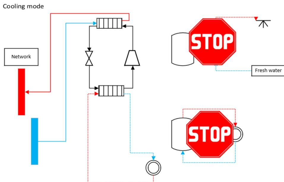
Figure 78 NTDH substation – reversible heat pump for SH/DHW and SC (cooling mode)
