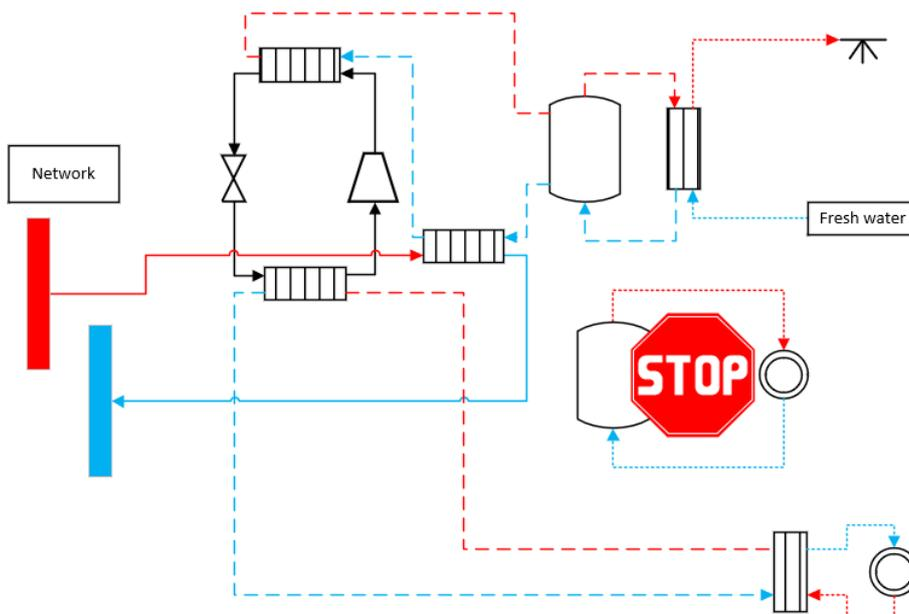
Figure 76 NTDH substation – BHP for DHW and SH, SC as heat source for DHW BHP (cooling mode)
