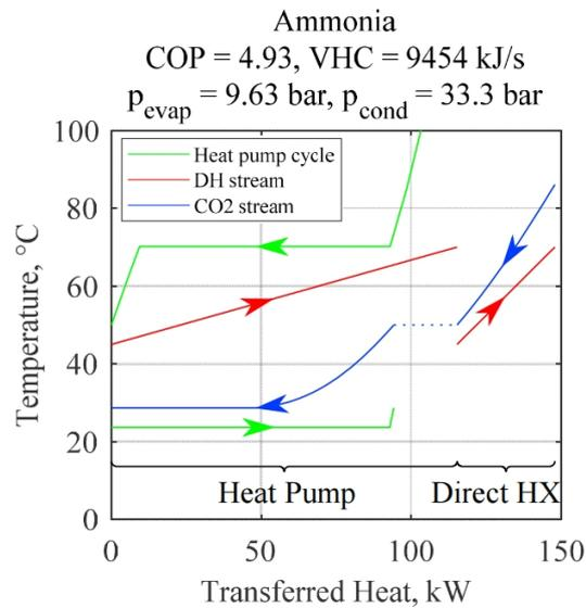
Figure 3: Temperature-heat diagram of an ammonia booster heat pump [18]
