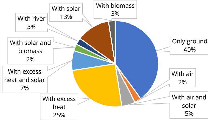
Figure 60 Overview of thermal sources coupled with ground in existing NTDH networks
