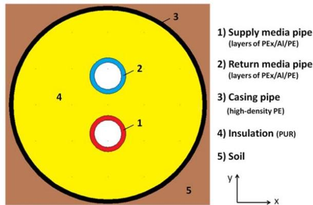
Figure 31 - Geometry and materials of a flexible, pre-insulated, twin pipe [42]
