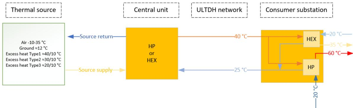
Figure 92 ULTDH network-based system with micro booster heat pump substation
