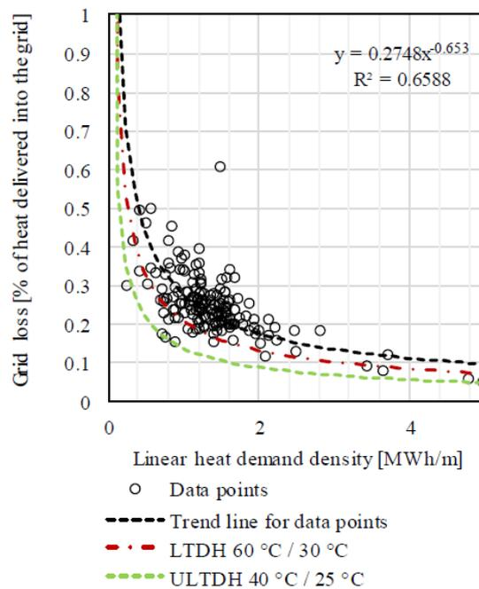
Figure 35 Correlation between heat demand density, DH temperature regimes and specific network thermal losses [4]
