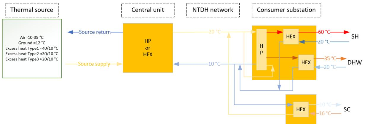
Figure 94 NTDH network-based system
