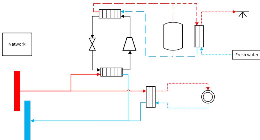
Figure 70 ULTDH substation – booster heat pump (supply only as heat source) and district heating storage unit
