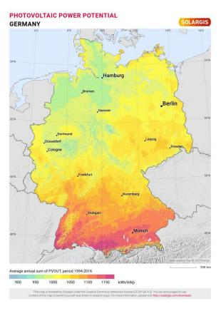
Figure 50 – Solar PV power potential in Germany (SOLARGIS, 2020).
