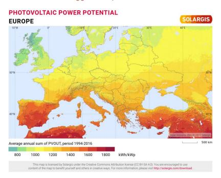
Figure 20 – Photovoltaic power potential in Europe (SOLARGIS, 2020).
