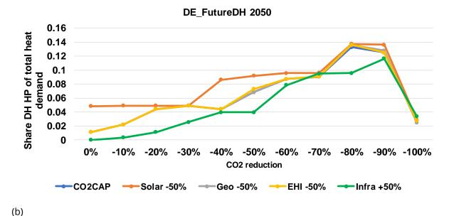
Figure 110 (a,b) – Shares of the LTH sources (upgraded by HP (heat pumps) in DH systems) in the total heat demand, as a function of CO<sub>2</sub> reduction level, as a result of LTH sources use and LTDH in Germany in 2050. Abbreviations: CO2CAP (CO<sub>2</sub> reduction level), Geo (Geothermal heat), EHI (Industrial EH), Infra (District heating infrastructure/ network cost)
