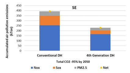
Figure 91 – The accumulated air pollutant emissions (NOx, SOx, PM2.5) attributed to heat supply in the heating sector of Sweden over the period 2020-2050 in the FutureDH and ConventionalDH scenarios (with 95% CO2 reduction by 2050).
