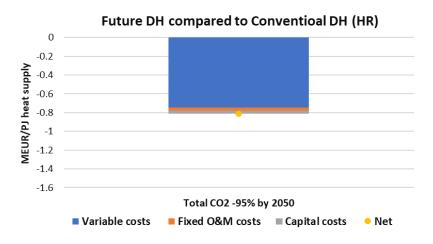
Figure 43 – The differences between the specific undiscounted Variable, Fixed O&M, and Capital (together with their total Net value) costs of heat supply in the heating sector of Croatia, averaged over the Years 2020-2050, in the FutureDH and ConventionalDH scenarios (with 95% CO2 reduction by 2050).
