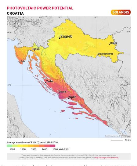
Figure 38 - The photovoltaic power potential in Croatia (SOLARGIS, 2020).
