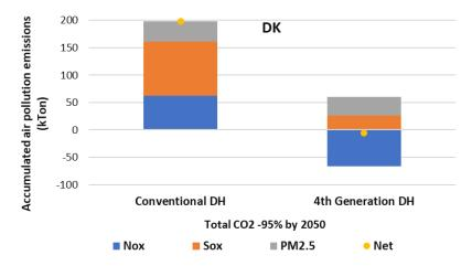
Figure 34 – The accumulated air pollutant emissions (NOx, SOx, PM2.5) attributed to heat supply in the heating sector of Denmark over the period 2020-2050 in the FutureDH and ConventionalDH scenarios (with 95% CO2 reduction by 2050).
