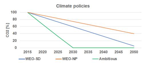
Figure 104 – Upper bounds for  $CO_2$  emissions in the model scenarios. Constraints apply both to fossil fuel  $CO_2$  emissions within the heating sector of the countries and to system-wide  $CO_2$  emissions when effects on electricity generation outside the modelled system are considered.
