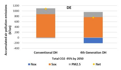
Figure 57 – The accumulated air pollutant emissions (NOx, SOx, PM2.5) attributed to heat supply in the heating sector of Germany over the period 2020-2050 in the FutureDH and ConventionalDH scenarios (with 95% CO2 reduction by 2050).
