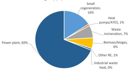
Figure 95 – District heating supply in Netherlands in 2013. The fuel used in power plant and in cogeneration is mainly natural gas, with a small share of coal and biomass (Niessink and Rösler, 2015).
