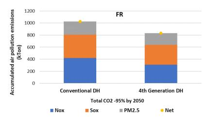
Figure 69 – The accumulated air pollutant emissions (NOx, SOx, PM2.5) attributed to heat supply in the heating sector of France over the period 2020-2050 in the FutureDH and ConventionalDH scenarios (with 95% CO2 reduction by 2050).
