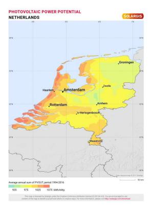
Figure 96 - Solar PV power potential for Netherlands (SOLARGIS, 2020).
